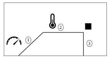
**Figure 2.** Representative scheme of application of thermal modification in the different treatments: 1 = time to reach the desired temperature (20 minutes for 120 °C; 30 minutes for 150 °C; 40 minutes for 180 °C; 80 minutes for 210 °C); 2 = constant temperature application period, 4 hours for all treatments; 3 = ending of treatment, removal of specimens from the oven and allocated in a desiccator to stabilize at ambient temperature, of approximately 20°C.
