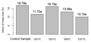
**Figure 4.** Mean of mass loss after the accelerated decay test of the juvenile *Handroathus chrysotrichus* wood, according to treatment.
