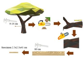
Figure 1. Representative scheme for obtaining the specimens of Ipe wood for the tests.
