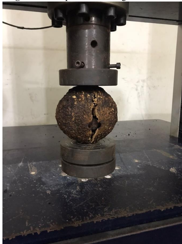
Figure 5. Compression testing of Brazil Nut
